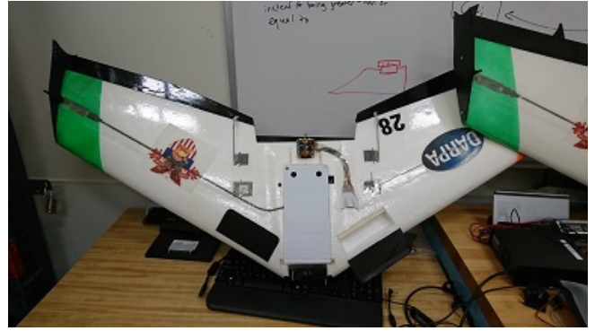
Fig. 1. Zephyr fixed-wing aircraft used in SASC swarm
