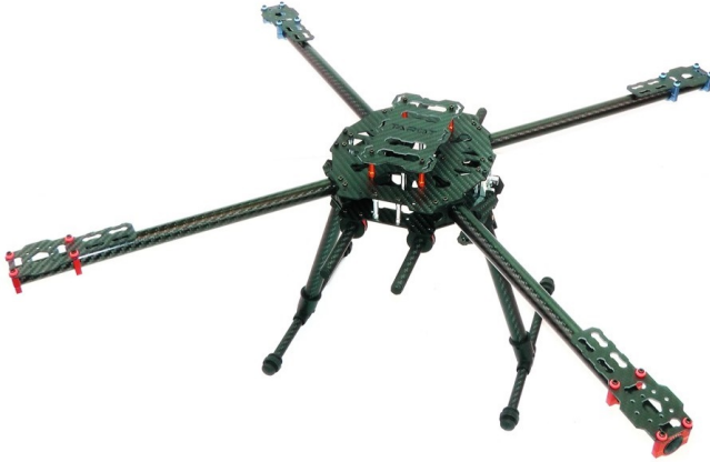
Fig. 4. Tarot Iron Man 650 frame used in our Variant 3 UAS design.
