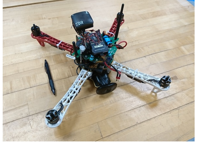
Fig. 2. Flamewheel F-450 quadrotor aircraft used in SASC swarm
